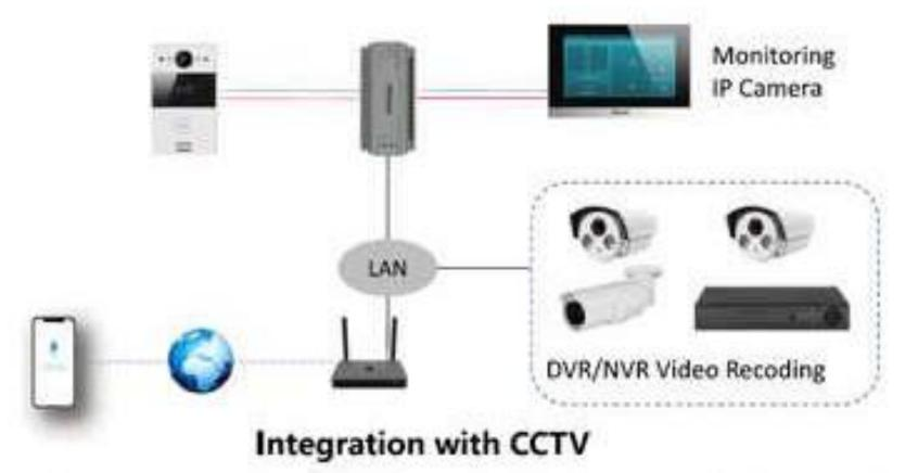
Akuvox 2-wire IP intercom system can be connected to general Ethernet and integrated with CCTV system
